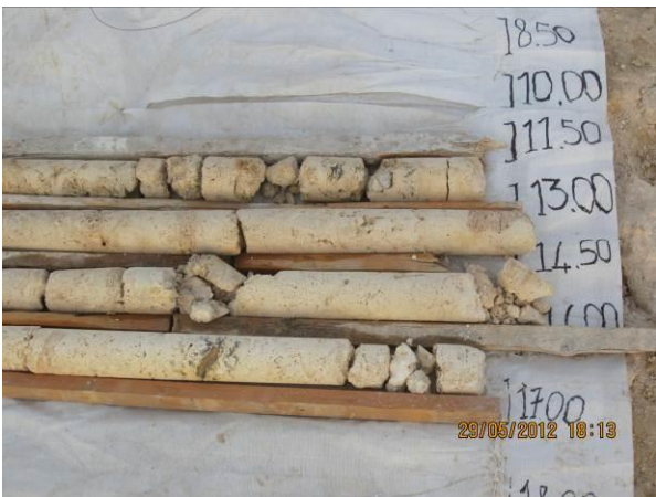
Figure 21 Results of a Drill Core after Injection
