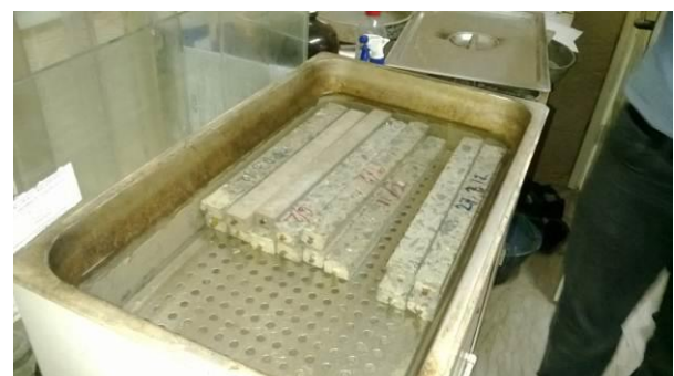
Figure 11 Sulfate test according to ASTM C1012, Test Blocks
