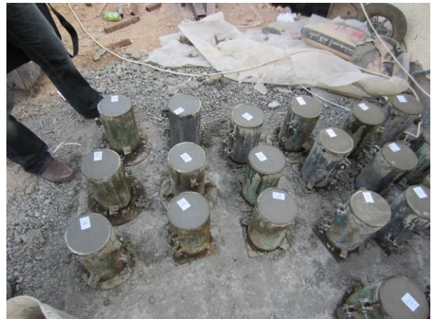
Figure 15 Test Cylinders out of Bored Pile Concrete
