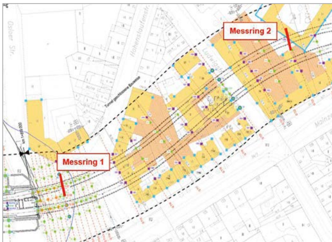
Bild 5 Geplante Lage der Messringe [1] Planned position of the measuring rings [1]
